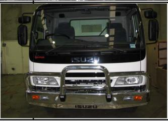
RAISE AND SECURE BULL BAR, LOCK BULL BAR IN PLACE USING THE TWO EYE BOLTS SUPPLIED. INSET TOW PIN INTO BAR
