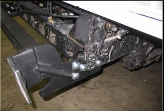
REMOVE BULLBAR BRACKET FROM BULLBAR
