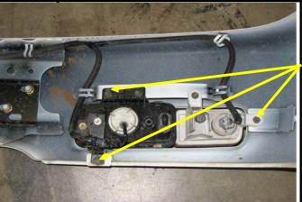
DISCONNECT WIRING HARNESS FROM LAMPS.
