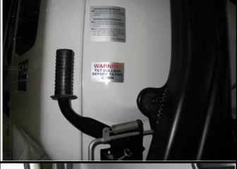
FIT WARNING LABEL TO BACK OF CAB NEAR CAB TILT LEVER.
