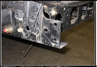
LOOSEN BOLT THAT HOLDS EARTH TERMINAL.
