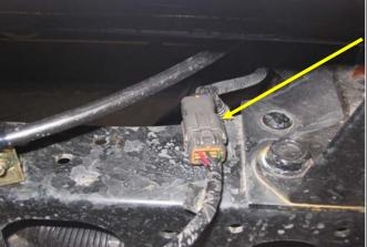
PLUG WIRING HARNESS BACK INTO MAIN HARNESS.
