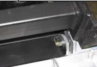
FIT BULL BAR MOUNT USING 2 x 9/16" BOLTS, 4 FLAT WASHERS AND 2 NYLOC NUTS.
